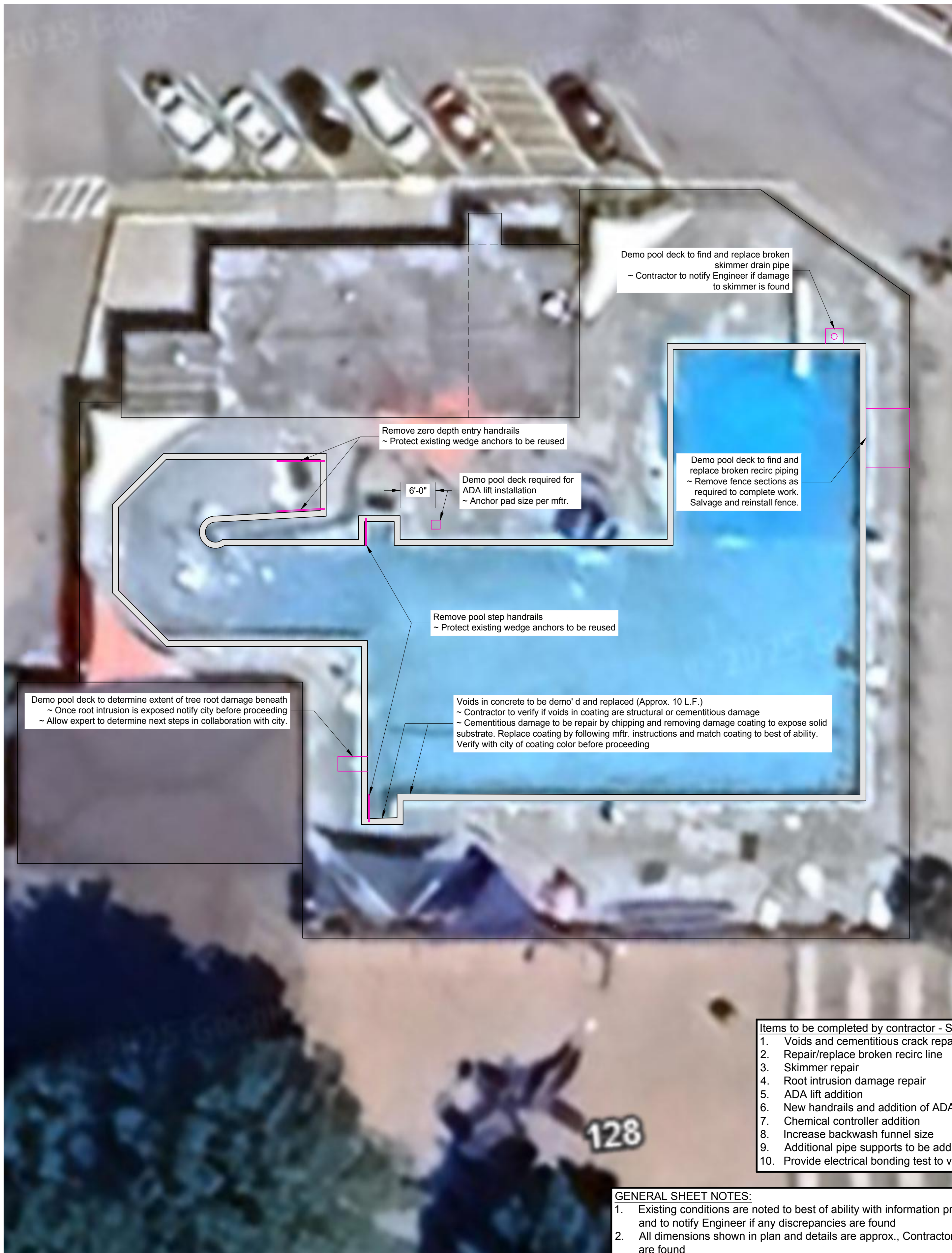
A POOL DEMO PLAN Scale: 3/32"=1'-0"
