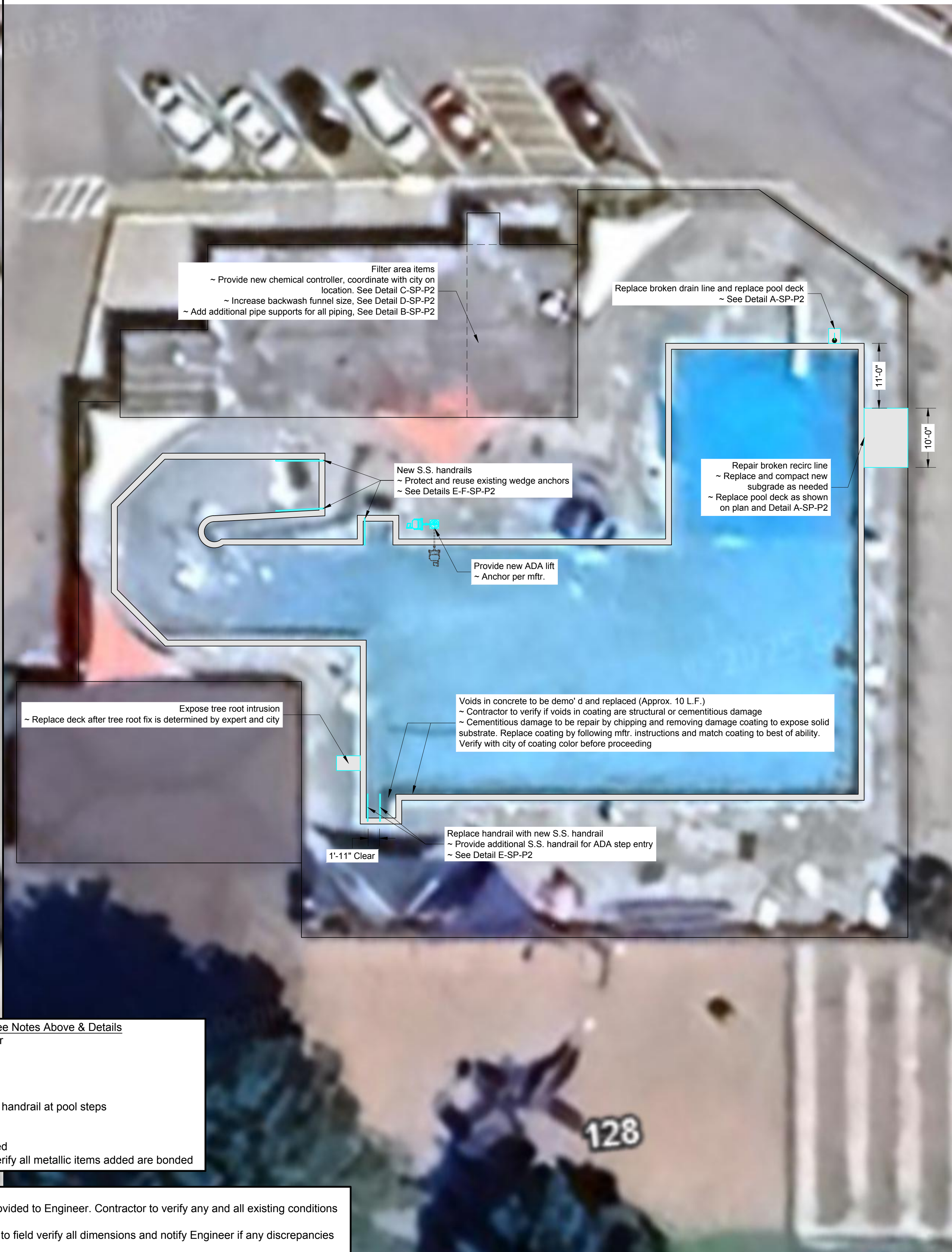
B POOL IMPROVEMENTS PLAN Scale: 3/32"=1'-0"
